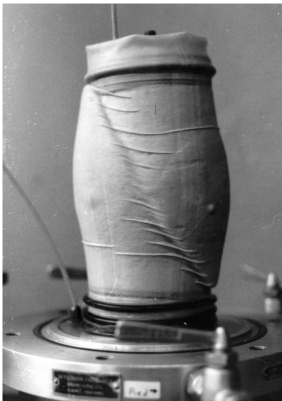
Fig. 1. Classical triaxial test specimen with shear plane; after J.L. Colliat-Dangus Doctoral Thesis, 1984 (Colliat-Dangus, 1986).
