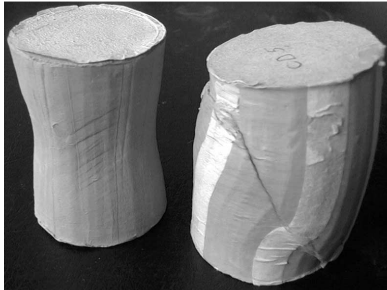
Fig. 5. Two clay specimens tested in axisymmetric triaxial conditions, one in compression (right) and the other in extension (left)—Photo J. Desrues.
